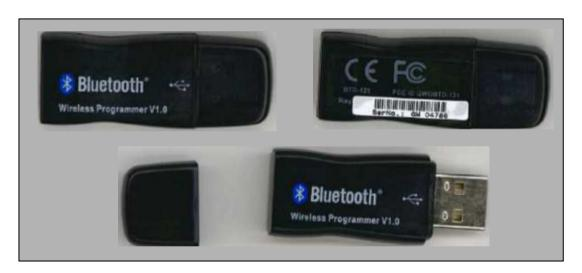
Attention: The serial numbers for ConnexxLink and the Bluetooth dongle are identical
